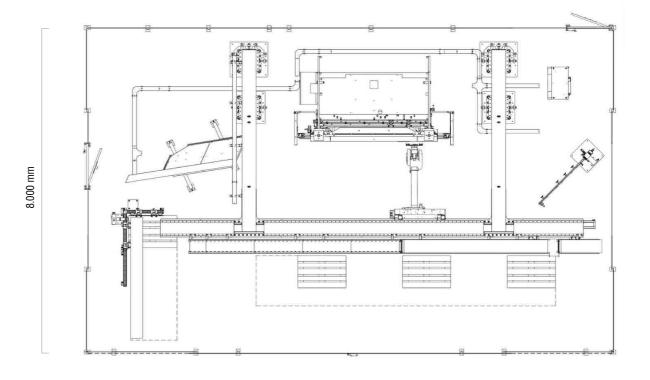
The TK MEGABEND CELL offers an advanced and versatile solution for automated bending needs, combining operational flexibility and space optimization to maximize the productivity and quality of production processes.
